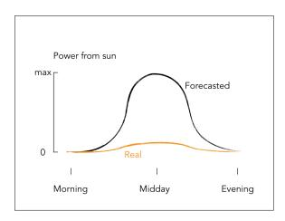
When a forecasted sunny day becomes a typical Belgian rainy day, the difference between the expected power production coming from the sun and the real production is significant.
