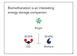
Several processes can be coupled to the storage system because they present interesting synergies. One of these processes is biomethanation. Since biogas has a large share of CO2, it is less energy intensive to recuperate and use in the carbon based fuels.
