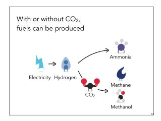
When storing electricity into fuels. Several options are available. The first step is generally water splitting and the production of hydrogen in an electrolyser.
