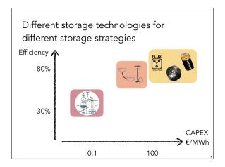
Another important comparison in addition to the previous slide is the roundtrip efficiency (from electricity stored to electricity retrieved) versus the investment per unit stored energy.
